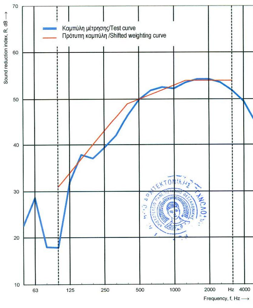
$$\begin{aligned} C_{50-3150} &= -6 \text{ dB} & C_{50-5000} &= -6 \text{ dB} & C_{100-5000} &= -5 \text{ dB} \\ C_{tr,50-3150} &= -15 \text{ dB} & C_{tr,50-5000} &= -15 \text{ dB} & C_{tr,100-5000} &= -13 \text{ dB} \end{aligned}$$
