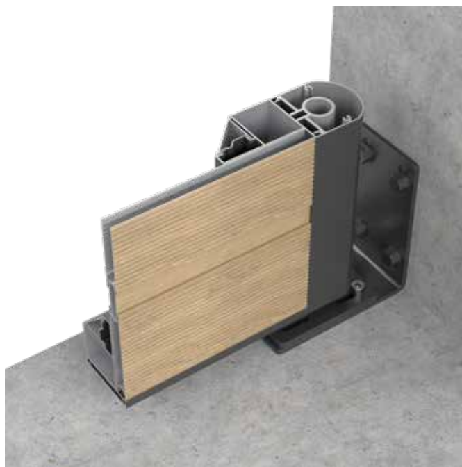
Detailed views of the sash and grooved profiles, along with the pivot axis profile with INOX 316 PIN able to hold 250 kg each. Maximum single door sash is close to 5m 2 withstanding a maximum weight of 80 Kg.
